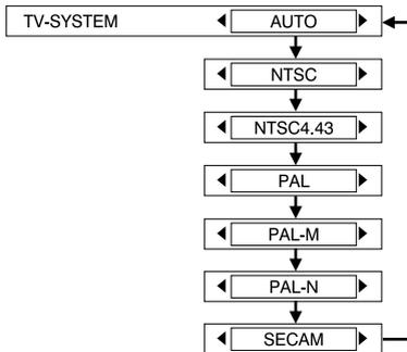
This should normally be set to “AUTO”. If the signal is of such poor quality that the correct format cannot be automatically distinguished, change the setting manually to the required TV system.
