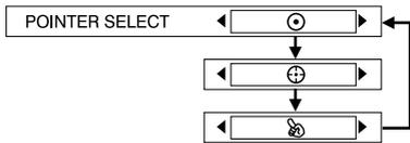
If you press the POINTER button on the remote control unit, the pointer will be displayed. You can select the pointer from 3 types as shown below (refer to page 35).
